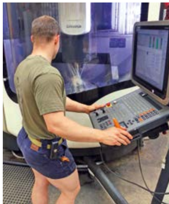
CPL J machining using a 5-axis CNC Mill
