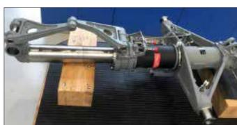
AMT Nose Landing Gear and C-17 Flight Loads analysis
