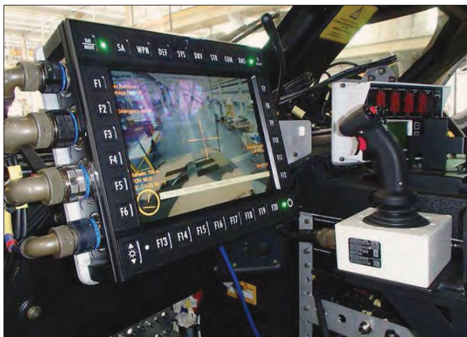
The RWS Display and Hand Controller.
