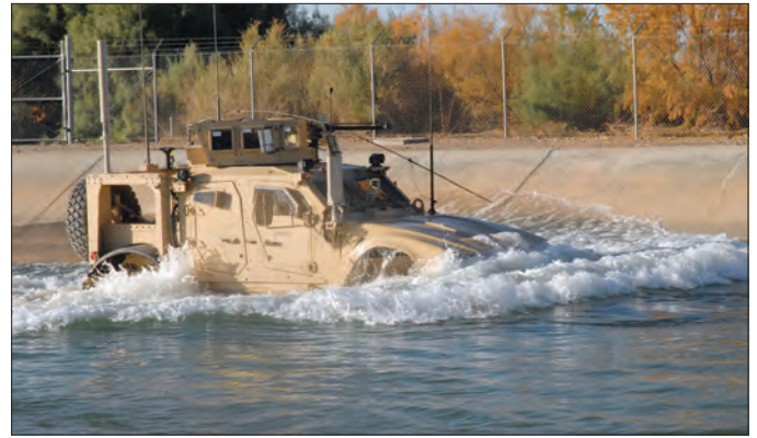
Combat vehicle water testing.
