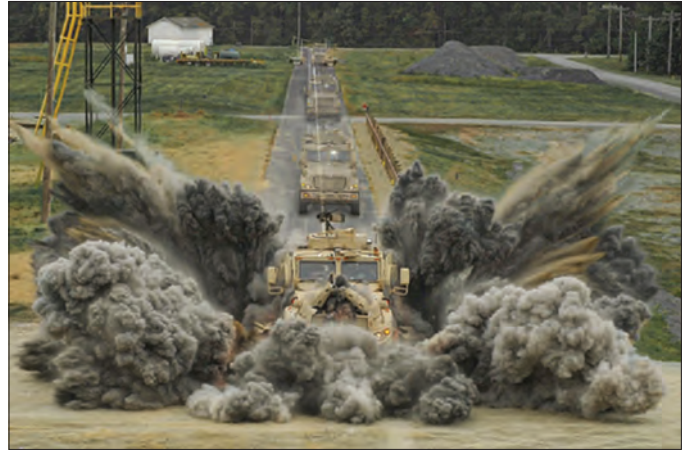
Sequenced photograph of a mine resistant vehicle undergoing dynamic rollover blast testing at Aberdeen Test Center.
