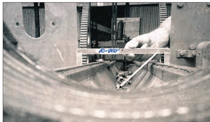
Gauge Minimum Cradle Width.
