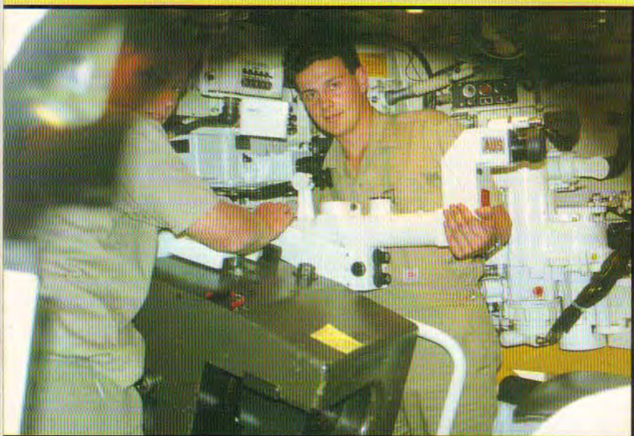
Centre L to R: CFN D. Hicks and CFN J. Claridge from the BLG fitting a Secondary Gunner's Sight to a Leopard Turret as part of their On-Job-Training program.
