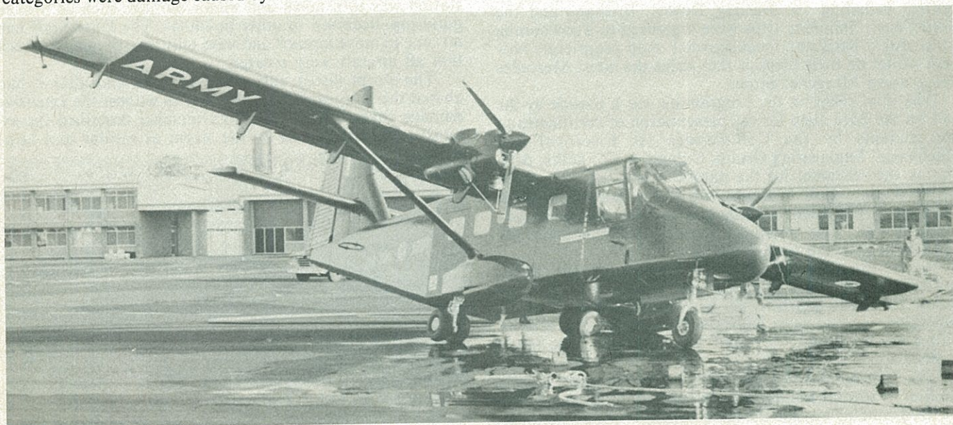
Nomad 306 with twisted undercarriage and extensive structural damage as a result of the winds.
