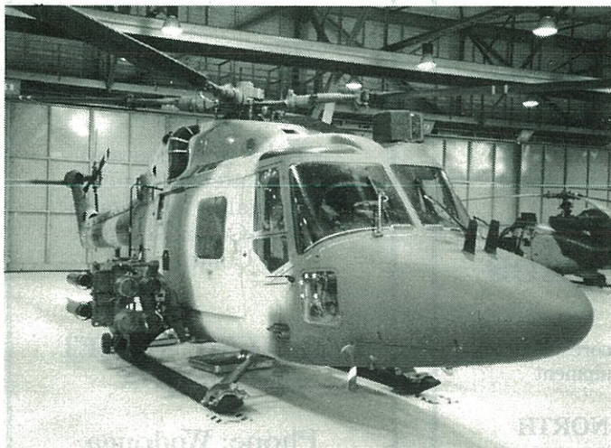
Lynx Mk2 - Tow missile system fitted. Tow missile sight on roof.
