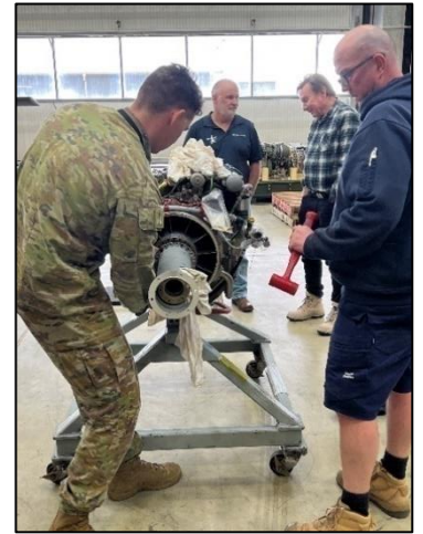
UH-60M engine being maintained off aircraft
