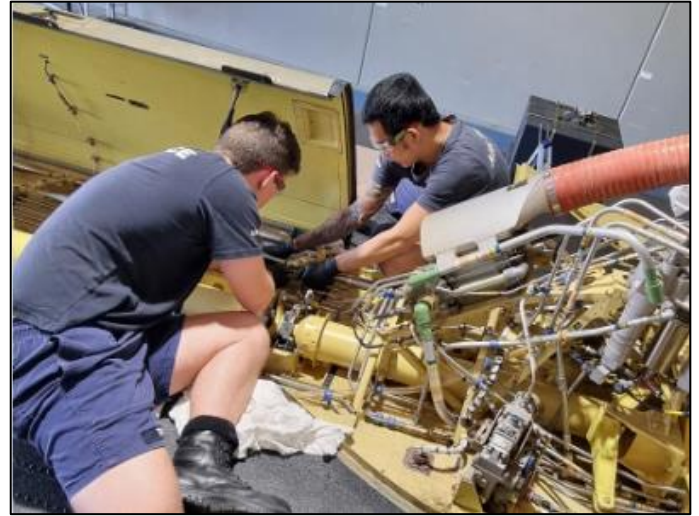
ASR LAC Malvin Johnson and AC Angus Trass conducting repairs on a CH-47F tunnel cover.
