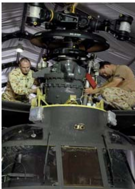
RAEME technicians guide the forward rotor assembly of a CH-47D during the aircraft reassembly in southern Afghanistan
