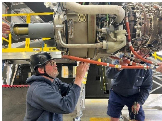
CH-47F Engine being maintained off aircraft
