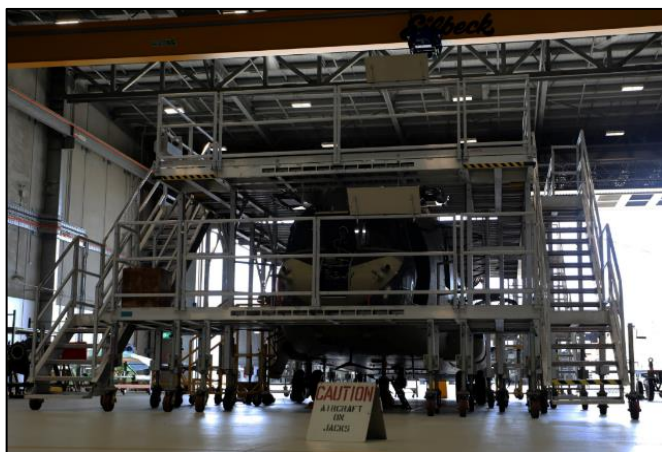
Chinook Surrounded by docking station, ready for service to begin
